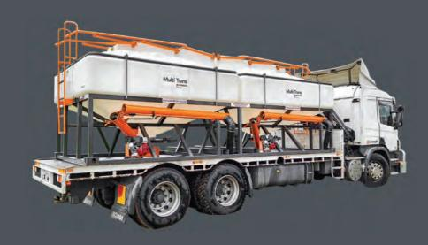
Suitable for liquid or dry goods transport 14m³ capacity per unit, 7m³ capacity per single pod Double bin unit - 6060mm long x 2430mm wide x 2400mm high
